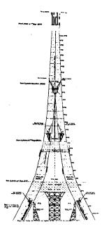
Fig. 1. Diagram of Eiffel's system of mobile cranes.
